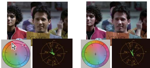
Rotating the outer ring of the color wheel (left) changes the hue angle (right).
